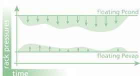
Operation with floating condensing and evaporation\* pressure to increase the efficiency and the performance of the compressor racks.
