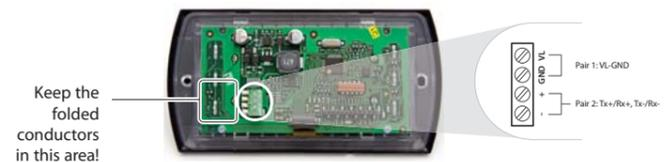
7. Finally, fix the pGD to the back piece folding the conductor only on the right side of the enclosure (front view)
