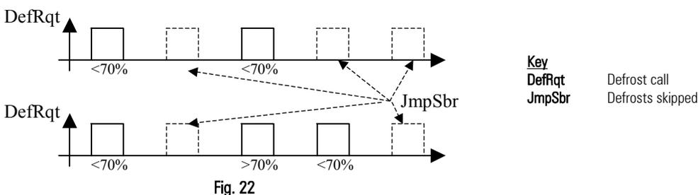
This function should be used with the programming of the defrosts equally distributed over the day (e.g. cyclical defrosts, parameter "d1").
