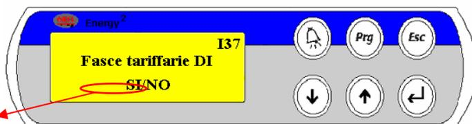
Enabling this parameter activates the functions of digital inputs ID 1 and ID2 for the change in rate band.
