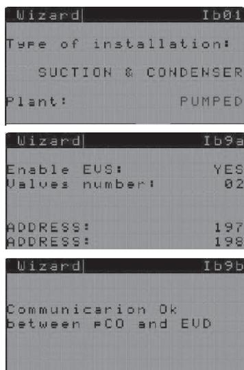
In this type of system, it is important to coordinate operation of the medium temperature rack with tube bundle evaporator control, to prevent low pressure problems. Pressure control inside the receiver is the main task; given the quantity of refrigerant contained and consequently its significant inertia, it is essential to activate the compressors based on the receiver pressure, and medium temperature rack suction pressure will only be monitored for safety, to prevent low pressure problems.
