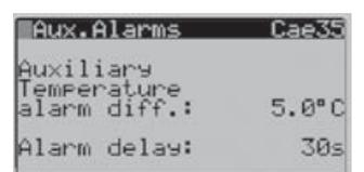
**Note:** when auxiliary control is enabled, it is recommended to also enable the prevent low suction pressure function, see paragraph 8.3.4 (prevent low suction pressure). In case of pumped systems, don't configure the second condensing line.
