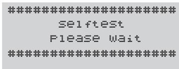
6. when this screen is displayed, wait 10 seconds and then release the buttons;
