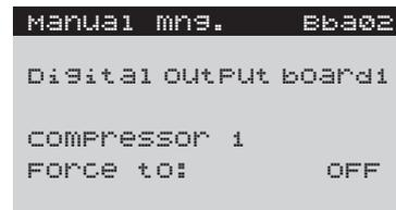
The output test is used to activate or deactivate the outputs (where necessary setting an output percentage for the analogue outputs), without observing any type of safety feature.
