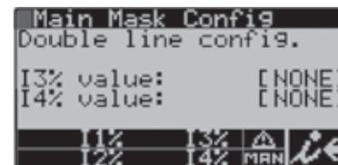
In configurations that feature control of two suction lines, 4 different percentages can be shown from the values described in the previous table. The customised main screen is simply an option that is available following configuration of the main screen in the Wizard.
