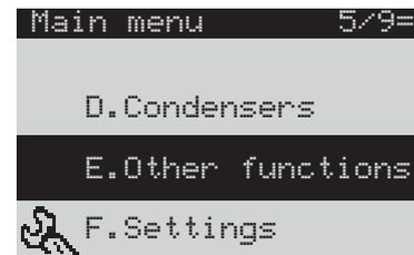
The top right corner shows the selected item and the current password level (for details see the following paragraph). The ↑ and ↓ buttons are used to select the desired menu item, while ← accesses the selected item.
