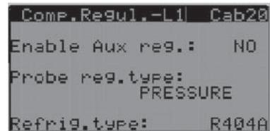
The function does not need to be enabled if "water chiller" is set in the installation Wizard
