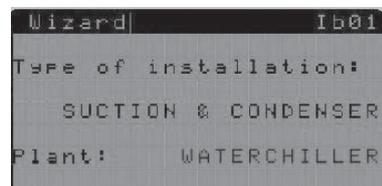
as auxiliary control by temperature probe is enabled automatically. Choosing a "pumped" system, on the other hand, automatically enables auxiliary control by pressure probe (see Appendix A.2)
