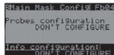
On this screen, users can choose whether to configure the part relating to the probes, or the bottom bar with the percentages or number of active peripherals in the circuit.
