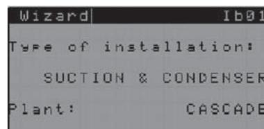
After having selected this type of configuration, the software takes a few seconds to pre-configure some settings relating to a typical cascade system, i.e. the second condenser line; the Wizard will prompt whether to
