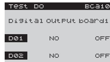
**Important:** manual mode and the output test can only be activated with the unit off.
