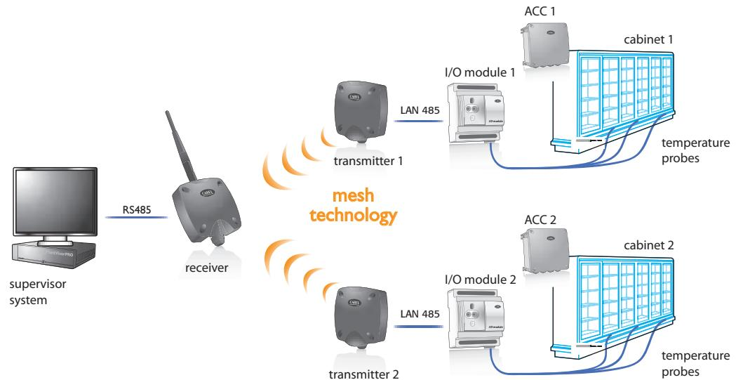
Globally, the installation is low impact (limited wiring, exploiting wireless technology, while retaining the controller already used on the refrigeration utilities).
