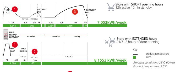
Double pull-down mode with priority on performance (FAST) or power consumption (ECO). ECO mode exploits machine-learning algorithms to calibrate pull-down duration in accordance with the requirements of standards in force. High temperature stability in conditions with frequent door openings.
