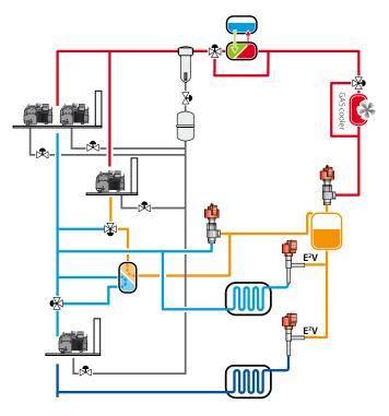
The liquid receiver normally works at around 35 barg (2°C) and the flash valve controls the pressure inside the receiver (safety valves calibrated at 60 bars).
