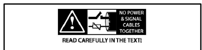
**WARNING:** separate the probe cables and the digital input cables as much as possible from the inductive load and power cables to prevent possible electro- magnetic interference. Never introduce power cables and signal cables (including those of electric control board) into the same cable troughs.
