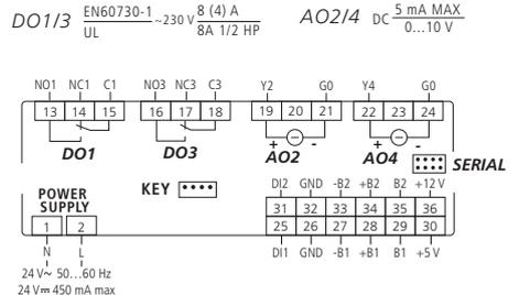
2.5 IR33/DN33 Universale with universal inputs - probe connections
