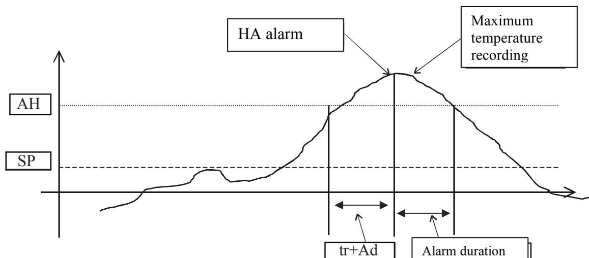
**"HF"** – this is activated after a power failure if, when power returns, the temperature is higher than the threshold represented by "AH" + "St". The following data are saved:
