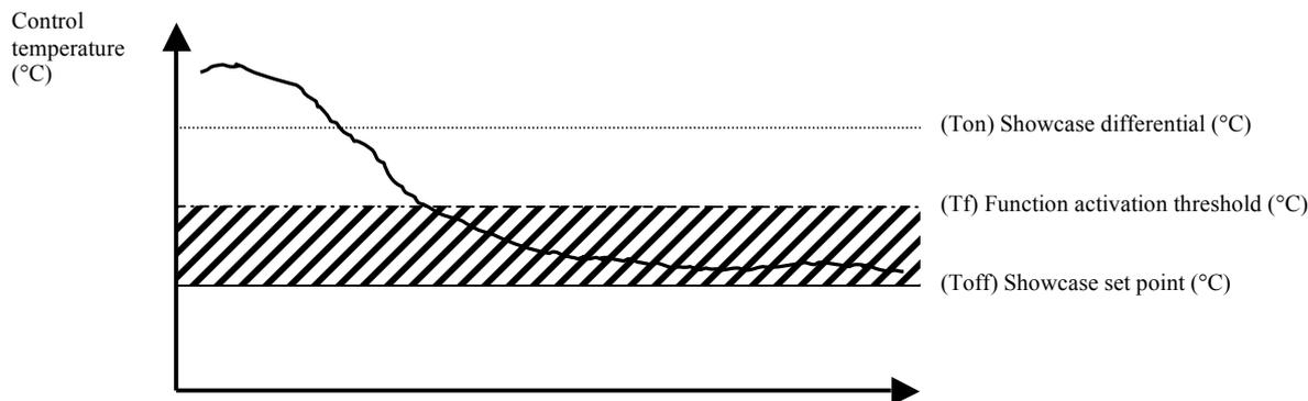
Function enabled with the optimum value of the parameter OSH. Except for sudden variations in the load or disturbance in the system, the showcase will remain in ON for a longer time than with traditional control, yet with a temperature and relative humidity that are much more stable and nearer to the set point.
