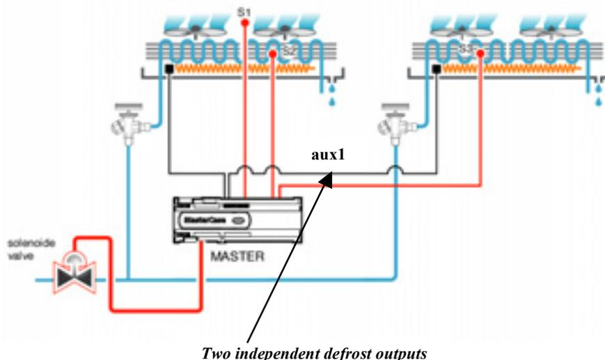
"H5"= 9, ON/OFF valve output (solenoid);
