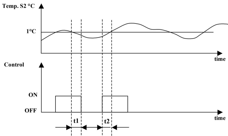
$$t1 + t2 + \dots tn \geq d3 \rightarrow \text{Start defrost}$$
