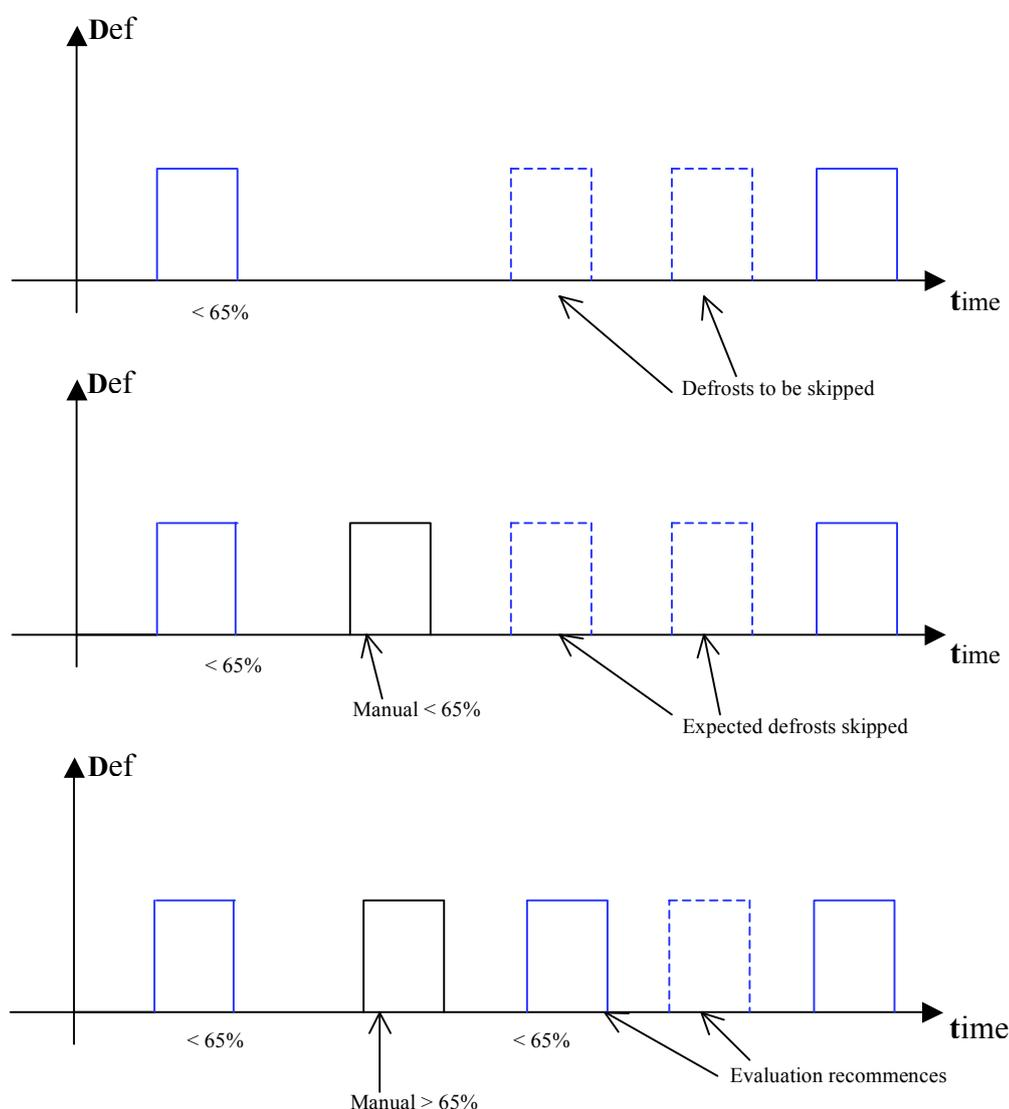
This function should be used with the programming of the defrosts equally distributed over the day (e.g. cyclical defrosts, parameter "dI"). This prevents skipping defrosts that would be the last before a long period programmed without defrosts (for example, when the clock is used to program the defrosting of the utility at night only).
