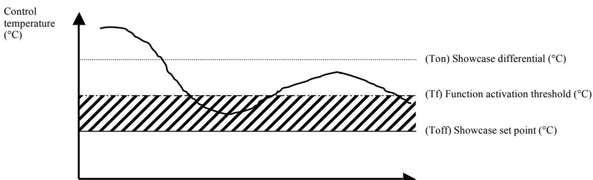
Function enabled with the value of the parameter OSH too high. The advantages of the function are not exploited adequately.
