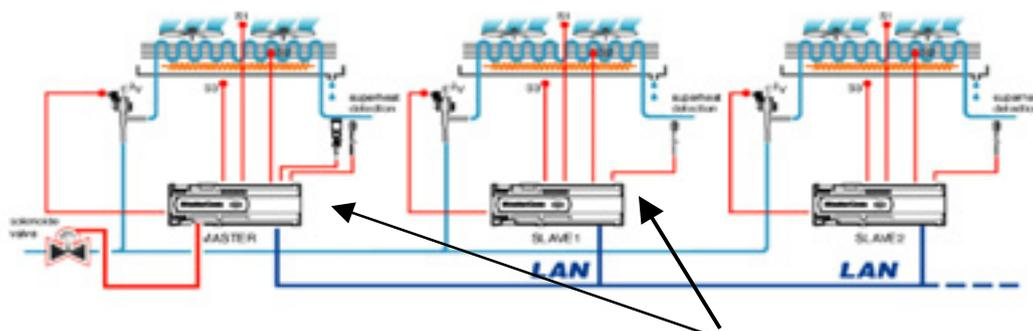
*Use of just one pressure probe propagated from the master to the slaves*
