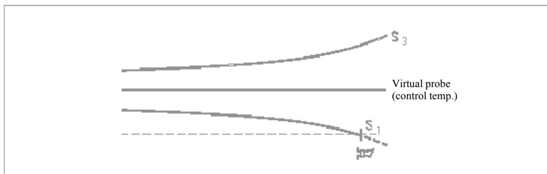
In this case, in fact, the temperature control is based on a "weighted" value of the two probes (S1 and S3). This means that despite the fact that the reference is constant, the temperature of the two probes may in reality differ significantly, with the risk of having an evaporator air outlet temperature (that is, the air that comes into contact with the product) that is dangerously low.
