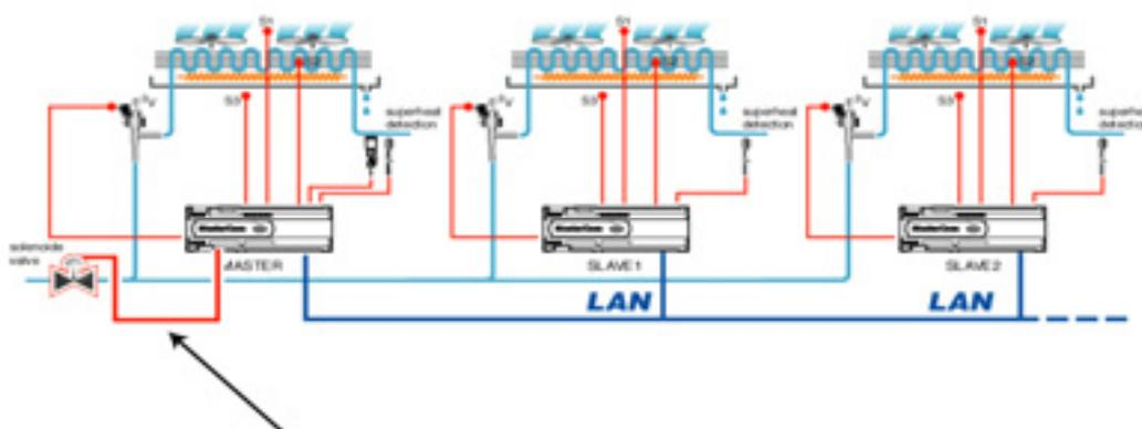
*Connection of the solenoid valve (or compressor) to the master only*
