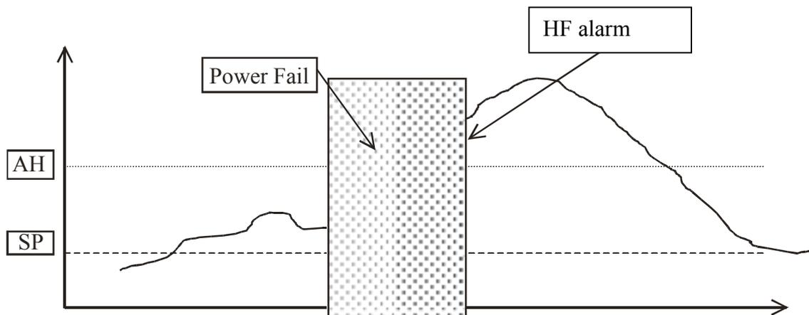
When an HA or HF alarm is activated, the display shows the codes "HA" or "HF", the alarm LED and the HACCP LED come on, the buzzer sounds and the alarm relay is activated.
