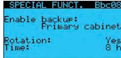
A system configured in this way will therefore comprise one cabinet that is operating and one in standby. The cabinet in standby will display "Off from backup" on the main screen if rotation is not enabled, or "Off from rotation" if awaiting the time set for rotation.
