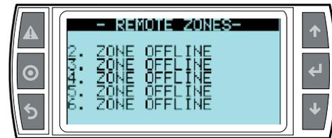
Indicates the current status of each remote location connected to the cabinet
