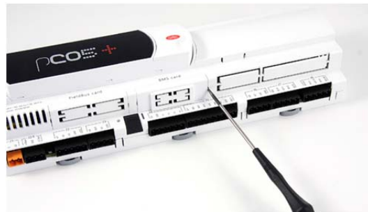
Figure 2.b - Removing the cover from the pCO controller
