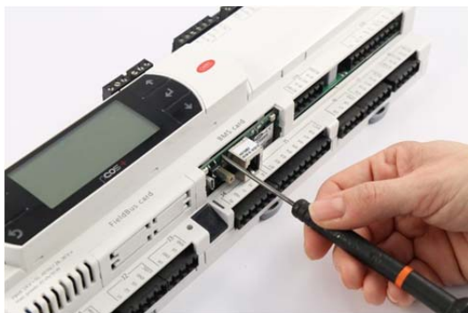
Figure 2.e – Removal of pCOWeb from controller
