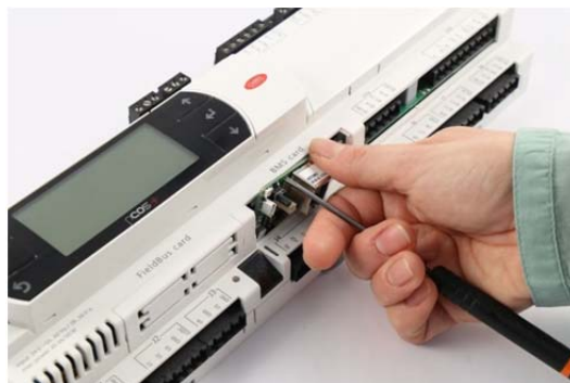
Figure 2.e – Removal of pCOWeb from controller
